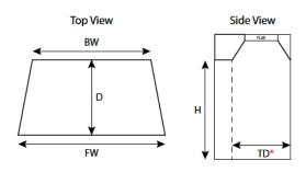
FW (Front Width): \_\_\_\_\_\_ BW (Back Width): \_\_\_\_\_ D (Depth): \_\_\_\_ H (Height): \_\_\_\_ TD (True Depth\*): ○ See-Through / Double-Sided Fireplace
